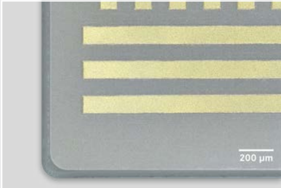
Cutting GaN and the geometrically accurate ablation of \mu\text{m} thick copper/gold coatings
