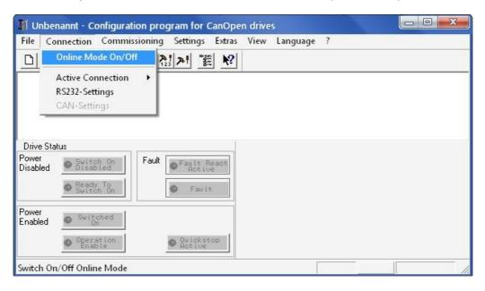
9. Do initial operation / parameterization IMDxx (refer to /1/ /2/) e.g. dialog window "Transmission" for setup encoder resolution, transmission ratio or feed constant:
