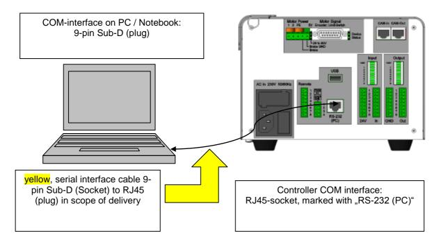
Image: Serial connection (RS-232) PC / Notebook with MC1 via interface cable
