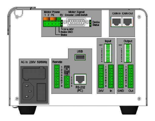
Image 3: Back side view controller MC1-10
