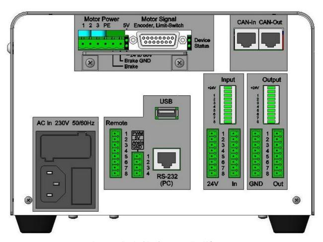
Image 4: Back side view controller MC1-20
