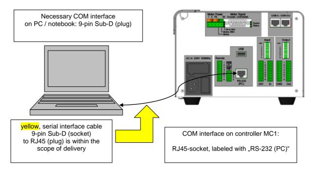
Image 6: Serial connection (RS232) via interface cable of PC / Notebook to MC1
