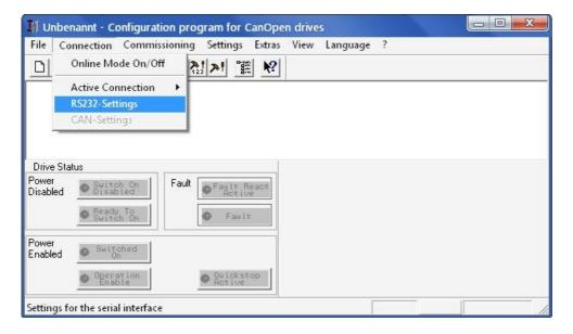
7. Set the used PC/Notebook COM interface (COM1...COM4) and baud rate to 57600 baud. Close settings dialog by clicking on button "Open COM Port":
