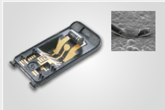
4. The metallized structures can then be assembled with components
