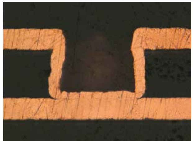
The result: perfect, reliable via plating
