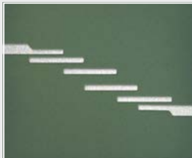
Then processing larger surfaces with milling technology (removing copper)
