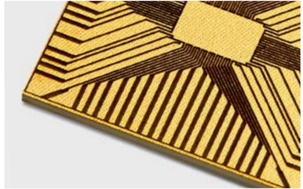
Ultra-fine structures on ceramic carrier material. No tool wear due to use of laser
