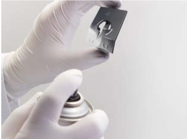
Coating 3D parts with LPKF ProtoPaint LDS
