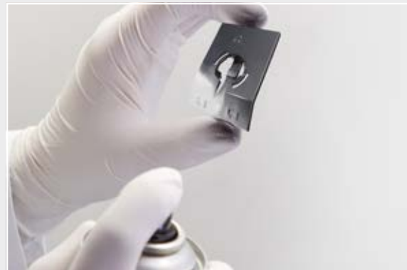
2. Painting the part with LPKF ProtoPaint LDS
