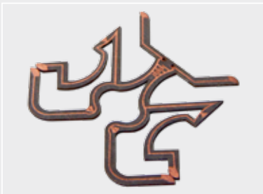
Microwave filter circuit sample structured and cut out on RO 5880 material
