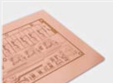
Laser-structured FR-4 boards feature high agreement between layout and actual geometry
