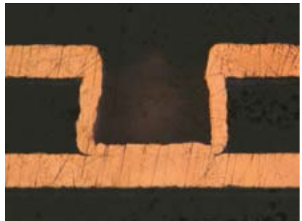
The result: perfect, reliable via plating
