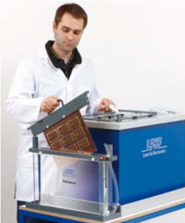
The additional LPKF ViaCleaner bath system cleans microvias in multilayer boards
