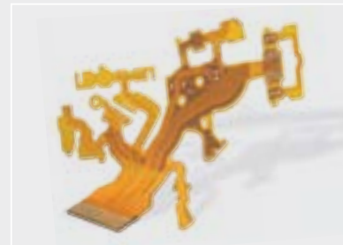
Accurate cuts in populated and unpopulated materials – even complex shapes: ceramics, polyimide and FR4
