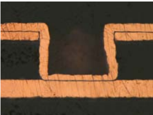
Without cleaning, the activator required for metallization forms a barrier
