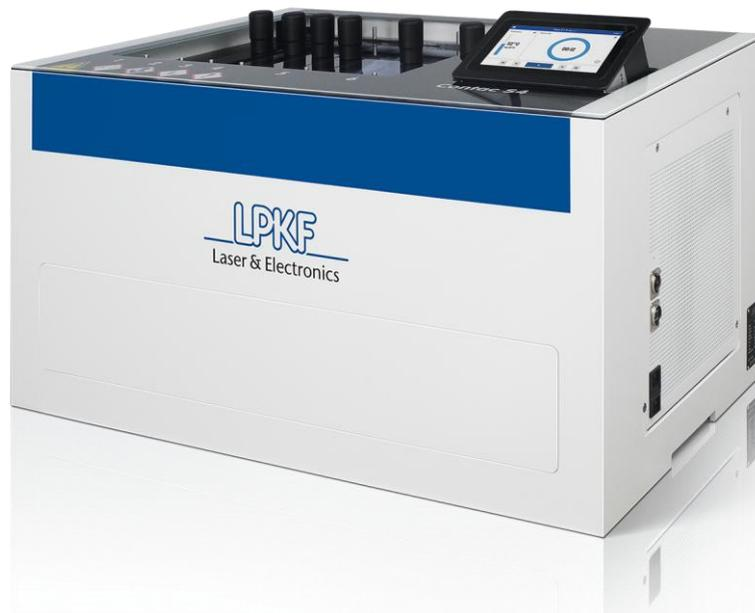
Complex electronic circuits have outgrown single-sided boards. The backs of the boards must also transmit current or signals; in addition, as complexity increases, the number of layers required also increases. Currently prototypes with up to eight layers can be produced in the lab. Various methods are available for connecting the layers.
