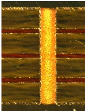
**The LPKF Contac S4 can be used for reliable, homogeneous through-hole plating of up to eight layers in the lab.**
