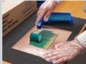
Applying the solder-resist lacquer
