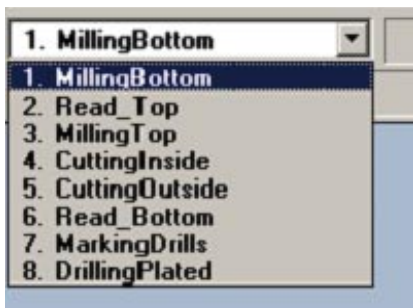
Process steps with LPKF BoardMaster
