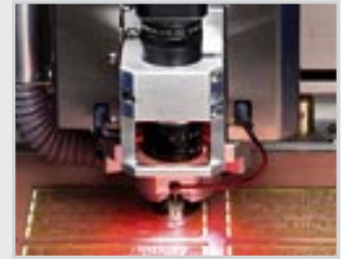
Drilling the board
