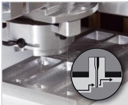
2 1/2-dimensional operation with Z-axis drive
