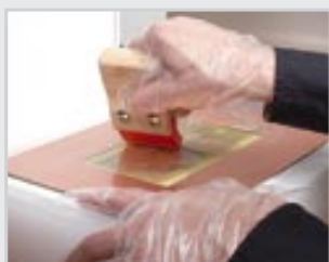
Using the squeegee to apply the conductor
