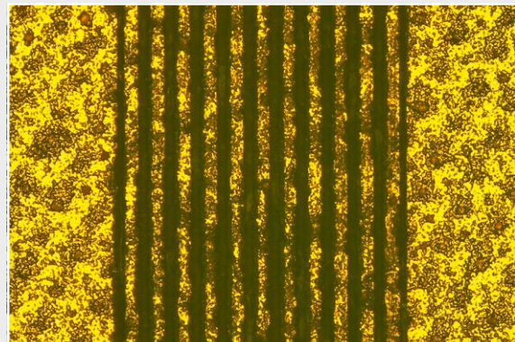
Structuring on Al 2 O 3 with Cu/Au plating using the laser with 50 µm/25 µm (line/space)
