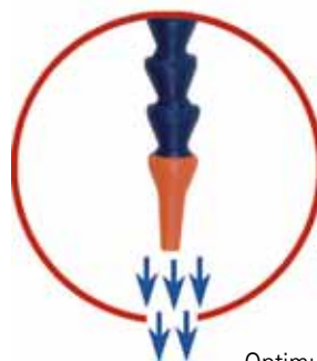
Diagram: CoolMin external with mating hose
