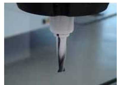
Tool, cooled by CoolMin internal
