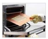
Curing the polymer in a hot-air oven
