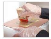
Using the squeegee to apply the conductor
