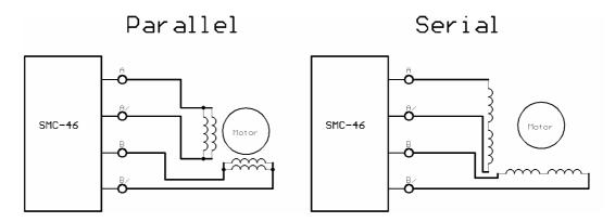
Refer to the data sheet of your stepper motor for the designations of your connecting cables. Check the connections carefully since a wrong connection can result in the output stage being destroyed.
