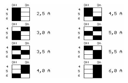
The set phase current is applied following power-up or after a reset (via pushbutton).
