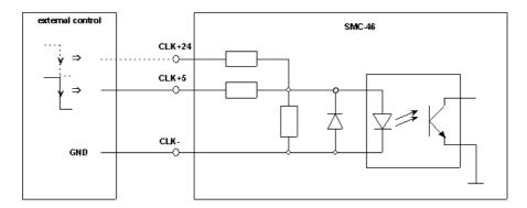
The phase current is stepped by one value on the falling edge of the Clock signal; the motor executes one step.
