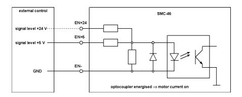
The motor current can be switched on and off with the help of the Enable input. The current values applied to the phases immediately before the current was switched off are fed to the phases when the current is switched back on. If the Enable input is not connected, the motor current is switched on and off by the Enable switch (see 1.4d).
