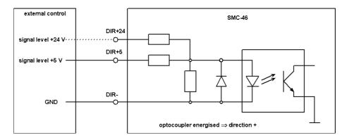
The Direction input determines the direction of motor rotation. There must be a pause of at least 5 µs between the time at which the direction of rotation is changed and enabling of the Clock input.
