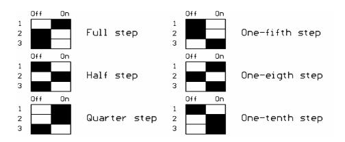
The set Stepping mode is applied following power-up or after a reset (via pushbutton).
