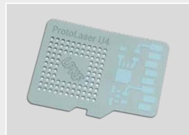
Delicate LTCC components: The UV laser can cut, engrave, and drill mechanically sensitive substrates.
