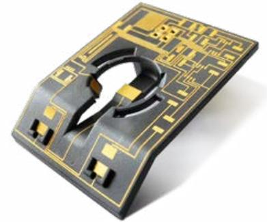
Laser Direct Structuring (LDS) is assuming a leading role for MIDs. A laser writes the conductive pattern on LDS-doped injection-molded parts. The traces are built up in a subsequent metallization bath.
