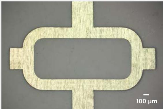
The USP laser can flexibly and precisely cut geometries out of thin metal foils. Thanks to the powerful CAM software, multiple trials can be made within a short period of time.
