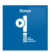
The status screen shows you all the relevant information at a glance. The progress of the program, the time remaining and the machine status are also visible from a distance.
