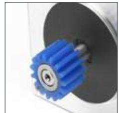
Pinions made of steel, aluminum or plastic can be mounted in various versions directly on the shaft. The motors can thereby be used as direct drives for gearboxes or rack and pinion drives.
