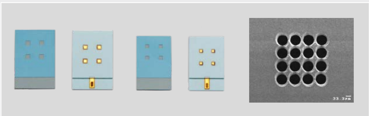
The UV laser cuts, engraves and drills mechanically sensitive substrates, such as LTCC components.
